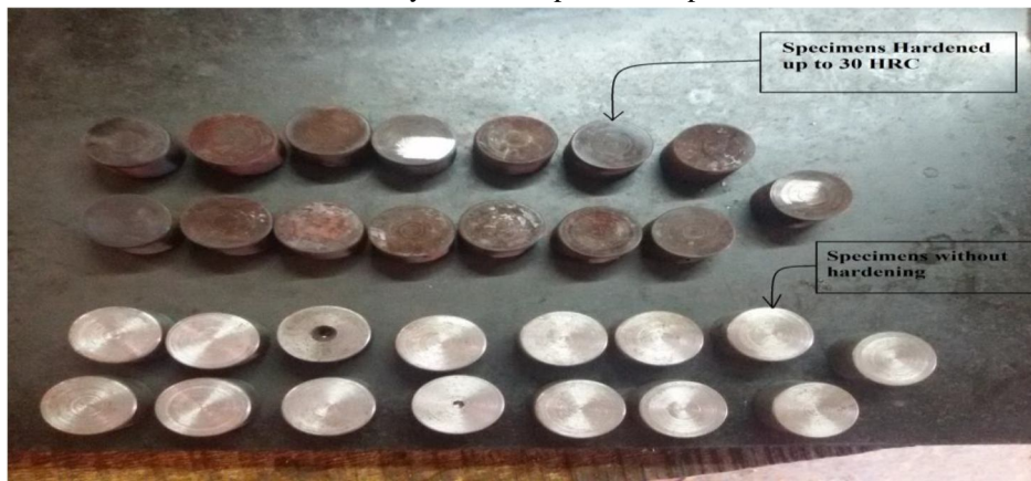
Fig 3.1.3 Specimens ready for machining on CNC
